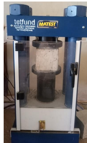
Plate2: Compressive strength test
