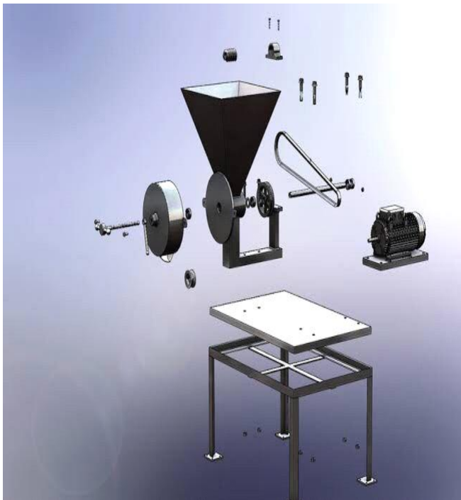
Plate 1: Exploded drawing of grinding machine
