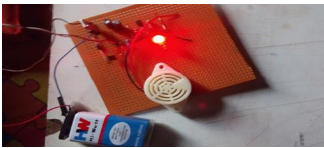
Fig. 4: Circuit on Veroboard in the Active Stage
